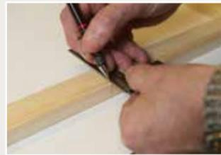
**4** Using a ruler, set square and pencil, measure and mark the halfway point along each side of the frame.
