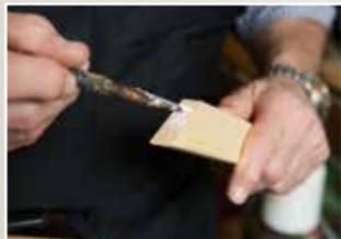
**2** Use PVA glue to the mitres before joining.
