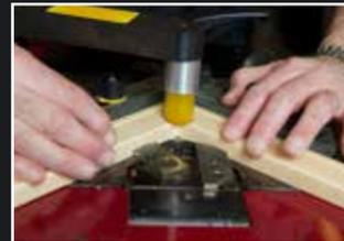
**3** Set up the underpinner to join frame. Position pins and wedges to join the corners of the frame.
