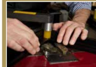
**12** Join the corners of the frame using an underpinner.
