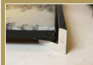
**11** Cut the floater frame moulding to length, ensuring you allow for spacing around the canvas edge.
