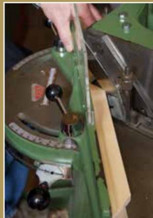
**1** Set Morso to required dimensions. Cut the stretcher moulding to make the frame around which the canvas will be stretched.
