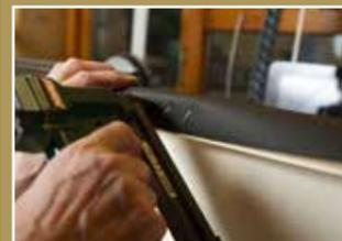
**8** Secure using a staple gun, working out from the centre point. Ensure the staples are inserted at an angle of 45 degrees. Use the stretcher plier to stretch the canvas around the frame to the reverse edge'.
